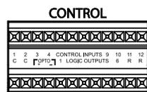
Used to connect switches or potentiometers, e.g. BLU-3 selector wallplate (Part no. Z-BLU-3). Looking at the control port connector (on the back of the unit), there are two common (ground) connections C to the left of the twelve CONTROL INPUTS and, two software assignable reference voltage outputs R to the right.
