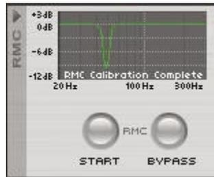
Double-clicking on the graph opens up an RMC window, which displays the precise frequency of the filter applied in each speaker by the RMC system, as well as its “Q” (bandwidth) and amount of gain reduction.
