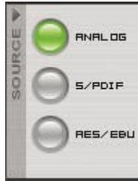
When changing input selection, signal is muted in all connected LSR4300 speakers for approximately 3 seconds to allow you to confirm your selection. The 3-second wait time can be bypassed and selection can be initiated immediately by pressing the INPUT button on the remote control or the speaker itself.
