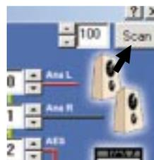
**3. Detect the EtherSound network** to determine the number of devices and inputs/outputs in the network, as well as their availability and their position. The management software supplied with EtherSound ES8in provides for one-click system detection. (Skip this step in case of manual set-up)
