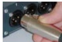
**2. Connect the analog audio sources and destinations to the EtherSound devices.** EtherSound ES8in/8out are equipped with XLR or terminal block connectors.
