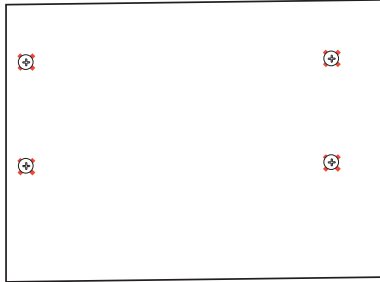
FIG. 6 Drill pilot holes and start screws, but do not tighten
